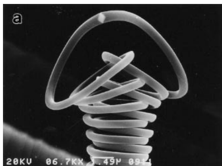
Fig. 8. Tip of the carbon microcoils. Arrow indicates a catalyst grain.
