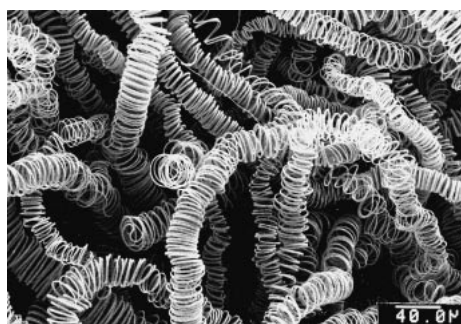
Fig. 5. Superelastic carbon microcoils with large coil diameter.
